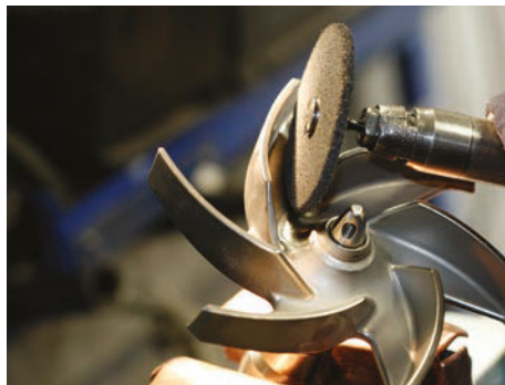
Finishing, maintaining and repairing turbine and propeller blades, without affecting their geometry.
