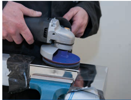
Prepolishing: ideal last step before mirror polishing.
