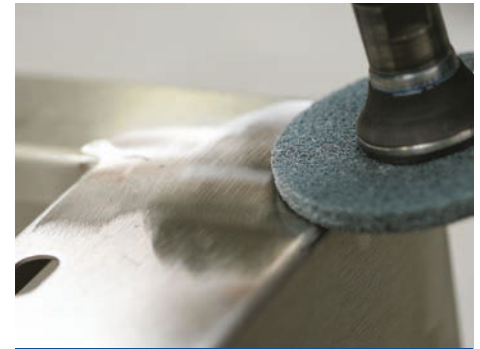
Improving surface roughness. Controlling the Ra value.
